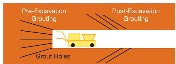
Figure 2: Pre- and Post-Excavation Grouting
