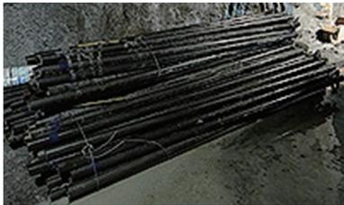
Figure 5: Stand-pipes (3 m Long)
