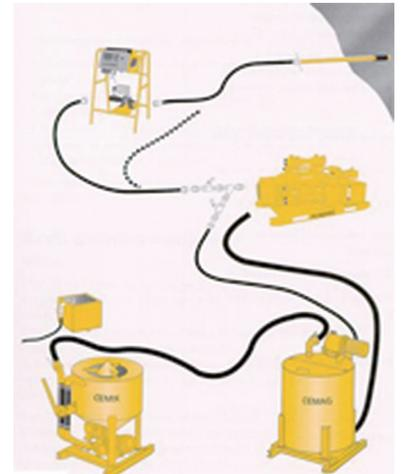
Figure 7: Grouting Equipment for One Grout Line
