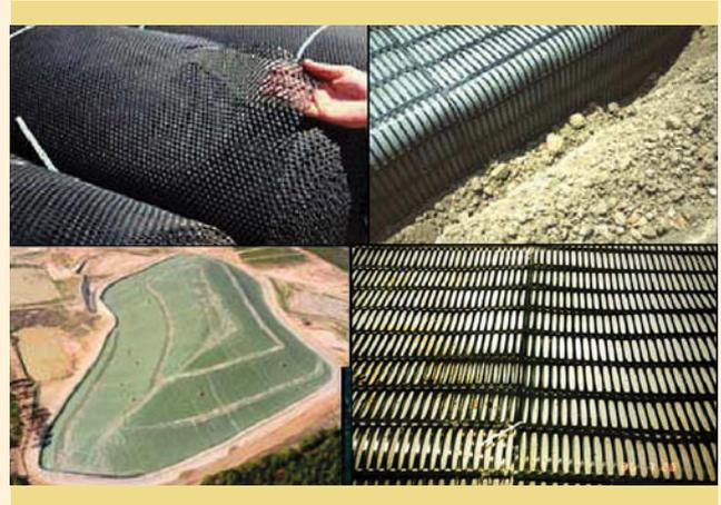
Dr Giroud further discussed slope stability and how this can be adversely affected by leachate recirculation and gas pressure. Waste slopes are more sensitive to a rise in pore water pressure than soil slopes due to their lower density. Geosynthetics are further less forgiving than granular drainage layers in terms of design and Dr Giroud recommends that a higher factor of safety be adopted accordingly.
